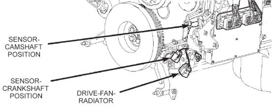
**2014-2019 Dodge 3.0L (EcoDiesel)** - Locate the engine crankshaft position sensor connector. This is located in the rear of the engine oil pan, just ahead of the transmission as shown in the picture. Tap the brown wire with light blue tracer (connector pin 3). Solder this connection and cover with heat shrink for longevity.
