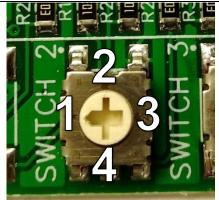
11. For Dodge 3.0L EcoDiesel and 2017+ 6.6L Duramax models, set "Switch 3" to position 2.
