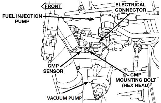
**IMPORTANT** The cam sensor plug on the BD harness must be connected the correct way around. Pay attention to the diagram below to ensure you connect the plug correctly. If this is connected backwards the high idle kit will not work and your tachometer may not work depending on model year.
