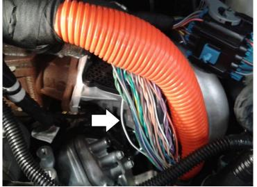
**2017-2021 GM L5P** – Locate the 8 pin sub-harness disconnect on the top of the engine for the crankshaft position sensor. Locate the solid green wire in pin 3. Remove some harness tape to have some wire to work with. Attach the light blue wire here for RPM pickup. Solder the wire and cover with heat shrink for longevity. Rewrap with tape when complete.
