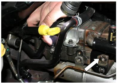
11.Remove the four bolts for the cooler and the nut that holds the transmission dip stick tube in place. Then nudge the tube out of the way to access the nut under the dip stick bracket.
