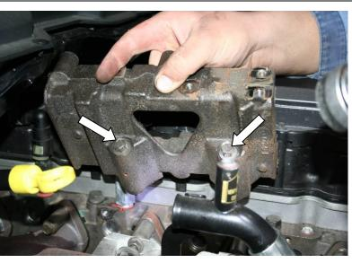
16.Remove the delta-P line bracket capscrew nuts and remove the delta-P line from the exhaust manifold and thermostat housing.
