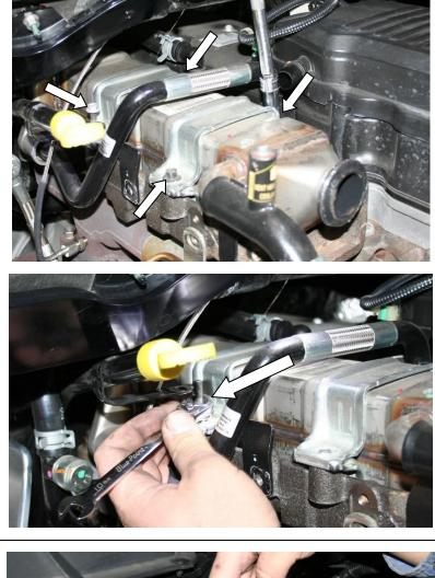
12.Remove the EGR coolant hose from the cylinder head to the cooler. (All bolts should be already removed) the hose is held in by orings. Remaining coolant will drip out.
