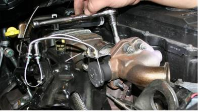
9.Remove the EGR flow direction valve from the vehicle.
