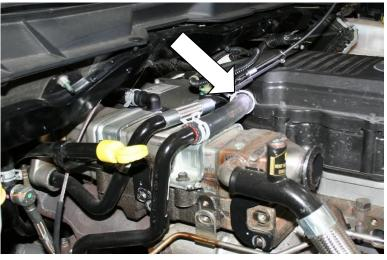
10.Remove the bolt that holds the CCV hose to the cooler then disconnect the clamp at the valve cover to remove the hose assembly.
