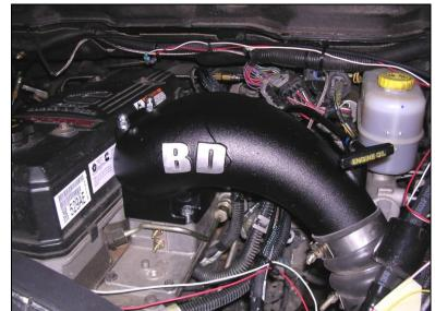
Move the intake around so that it is not touching anything and secure the intake with the supplied nuts. Note that the 12mm JIS nuts should be mounted to the smaller studs on the driver's side of the intake, while the 13mm Acorn nuts should be mounted to the longer studs. Be sure to place the washers underneath the Acorn nuts.
