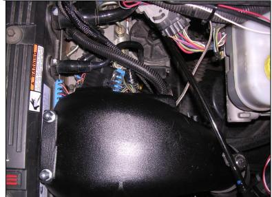
You can now reconnect the factory silicone boot and clamp. Be sure to clean the inside of the silicone boot with either a non oil based electrical contact cleaner or brake clean.
