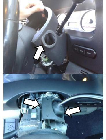
Using a punch and a hammer, drive the "press in pin" out of the shifter assembly. This will allow the shifter handle to be removed from the vehicle.
