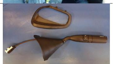
Install the new shift lever into the shift lever adapter. Slide the boot back on the shift lever to allow access to the mounting screw.
