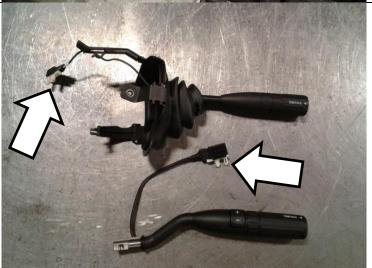
16. Remove the boot from the old shift lever and transfer to the new one. The boot will have to be stretched to fit over the electrical connector.
