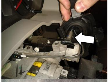
15. Remove and discard the white plastic securing clip from both the old and new shift lever electrical connectors to make boot transfer easier.
