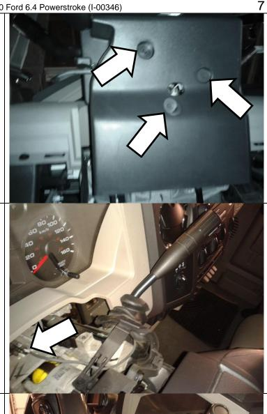
Pop the electrical connector for the *12.* shift lever out of the mounting location on the top of the steering column. Disconnect the shift lever wire from the vehicle.
