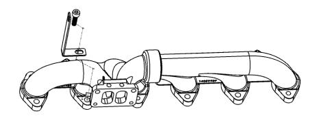
You now have the option to drill a hole through the OEM coolant pipe tab and secure the brackets together using the 1/4 (1100110),1/4" flat washer (1100111), 1/4" lock washer (1100112),and the 1/4" nut (1100113) supplied. Use a 5/16" drill bit to accomplish this.
