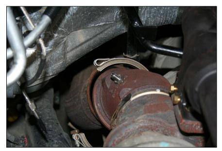
Disconnect the compressor outlet boot.
