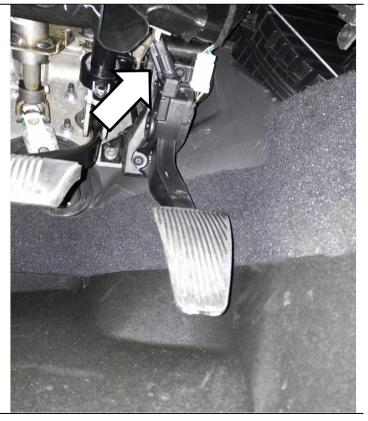
Plug the TSBooster in to the pedal and then into the factory wiring harness. Ensure both connectors click into place to confirm they have latched.
