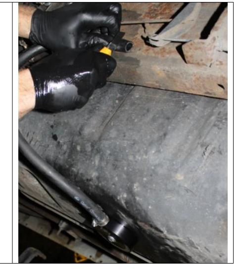
12. Now run your fuel line to the lift pump and cut to length. Secure the hose at both ends with the supplied gear hose clamps.
