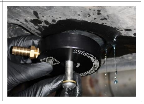
10. Turn the bolt by hand until the sump bottoms out on the tank base.
