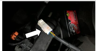
10. Route the BD harness towards the brake hydro-booster. Disconnect the two wire master cylinder pressure switch. The connector is on the bottom of the master cylinder.
