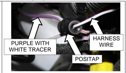
Install push button switch and connect to the BD wiring harness.
