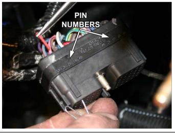
The two wire leads from the exhaust brake control harness (with the ECM pins precrimped) can now be plugged into the ECM. Insert the tan wire into Pin #39, and the black wire to Pin #42. They should snap into place. Once this is complete, you can re-install the ECM plug. Secure the wiring loom using the supplied tie wraps.
