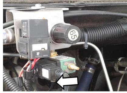
Connect the main ground connection to the body ground on the passenger side of the engine bay near the regulator assembly.
