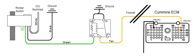
This switch relay is **not required** when wiring the exhaust brake with the push-pull style switch.
