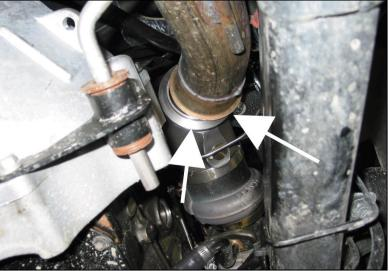
Tighten all clamps that secure the brake to the flanges.
