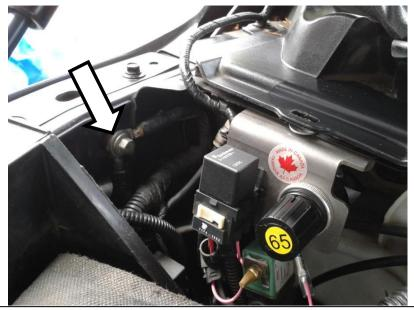
Connect the main power feed to the passenger side positive battery terminal clamp. This is the red wire with a ring terminal installed on the end.
