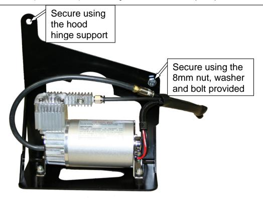
Feed the compressor air lines and wire through the fender into the engine bay, they will be connected later. Lift the compressor into place.
