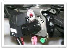
**NOTE**: Over the next two weeks, the backpressure at idle may rise due to initial carbon build up on the inside of the brake housing and on the butterfly. The stop bolt may need to be adjusted again to compensate.
