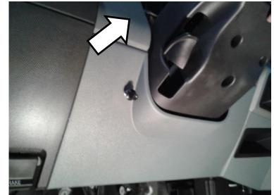
12. Drill a 7/8" hole in the dashboard with a stepper bit or hole-saw. Using a small file, create a notch for the locator tab of the switch. Clean up the edges of the hole as necessary with the file.
