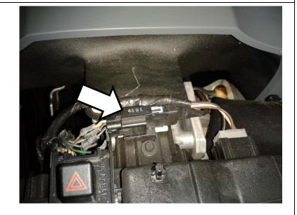
8. Use wire ties to secure the wire down the bottom of the steering column beside the OE harness.
