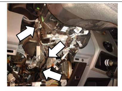
9. Remove the two 7mm screws securing the OBD connector below the dash.
