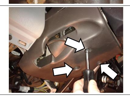
6. Pull the steering column covers apart and remove top cover.
