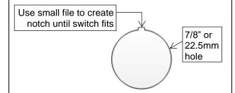
Install supplied switch decal onto the dash aligning the notch on the decal with the notch you created. Then install the switch into the hole.
