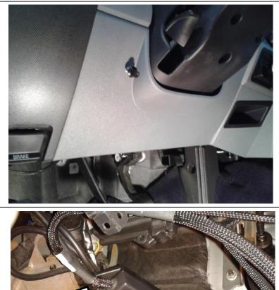
5. Remove the three 5.5mm screws from the bottom of the steering column cover.
