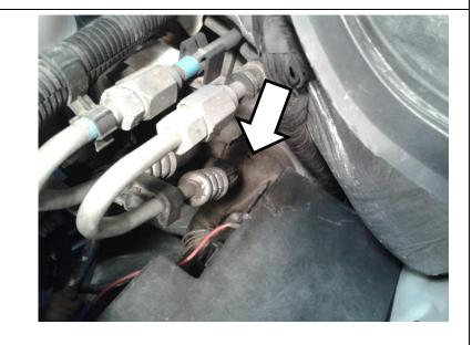
16. Connect the engine bay wiring disconnect to the in-cab wiring harness.
