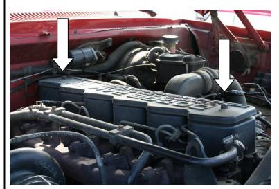
2. Using a **15mm** socket remove each of the valve covers.
