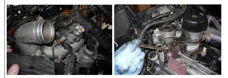
12. Reinstall the oil filter and EGR valve, service both as required.
