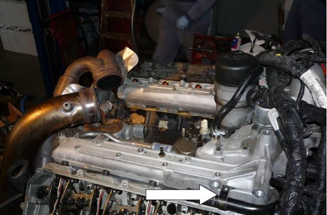
U.S. Shipping Address: 1124 Fir Avenue, Blaine, WA 98230 U.S. Mailing Address: P.O. Box 231, Sumas, WA 98295 Phone: 604-853-6096 | Fax: 604-853-8749 | Internet: www.bddiesel.com NOTE: Bend back the tab on the rigid metal tube at the RH side of intake manifold to allow manifold to clear.
