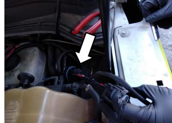
Under the truck, locate the transmission connector. Rotate the lock ring counter clockwise to release it.
