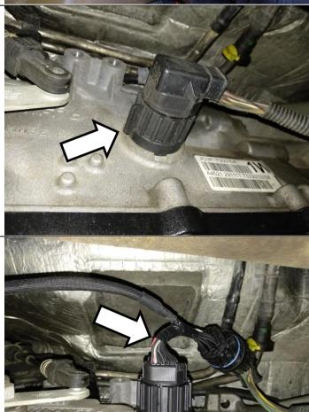
Route the supplied BD harness to the transmission and connect it inline.
