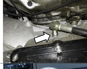
Stock pressure will range between approx. 70-170psi. With the BD kit installed the pressure is boosted up to 300 psi at higher engine load (15 psi+turbo boost).
