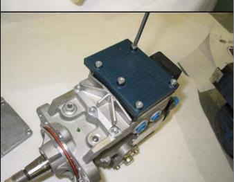
Screw in the retaining screws until they are snug. **Do not over-tighten them**.
