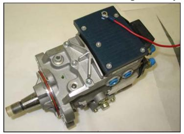
Strip both ends of the supplied 14-gauge red wire (*P/N# 1607412*) and crimp on the supplied eyelet connector (*P/N# 1300100*). Place the eyelet connector over the Piercing Allen Screw and start the lock nut (*1200307*) onto the Allen screw. Decide the best direction for the wire then tighten the lock nut down using a 3/8" wrench while securing the Allen screw with the Allen key.
