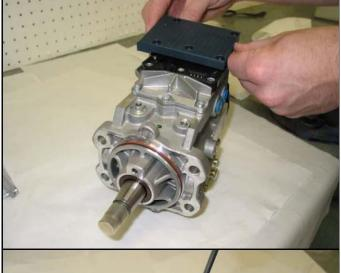
Place the plastic cover supplied in the kit on top of the pump, with the flat side up and lining up the holes for the 5 retaining screws.
