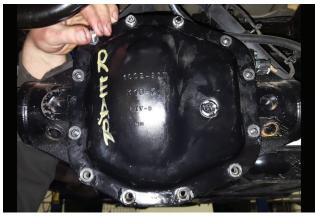
Place drain pan under rear differential where it can catch fluid. Remove factory plug and allow fluid to drain. Then remove bolts (x12) and differential cover.
