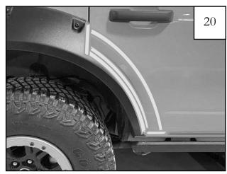
Mask off the areas surrounding where the red tape liner on back of the rear door inner bracket will contact the door surface.
