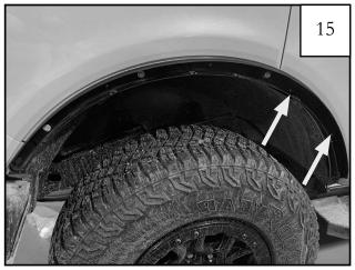
Use (2) SW1-0008 bolts, (4) WA1-0015 washers, and (2) NU1-0016 nuts to complete bracket installation. (See diagram Step 16)
