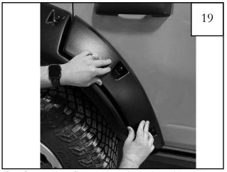
Test fit rear door flare assembly in place. Note where the red tape liner aligns with the edge of the door.
