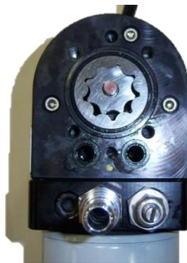
**STEP 7:** Install the Gerotor Cap. Be very careful not to dislodge or pinch the O-rings.
