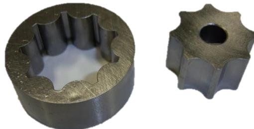
**STEP 4:** Remove the O-rings and clean/inspect the inside of the Gerotor pocket.
