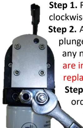
**Step 1.** Remove the regulator by turning the Adjustment Screw counter-clockwise using a 3/4 wrench.
