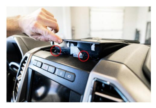
6. With the tray unclipped, pull the top of the radio display trim towards you, until it unclips. There are multiple clips that will need to release, take your time as you do not want to damage the trim piece.
