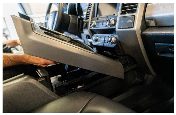
2. Once the trim piece is removed, locate the (2) T20 torx screws as shown below, and remove them.
