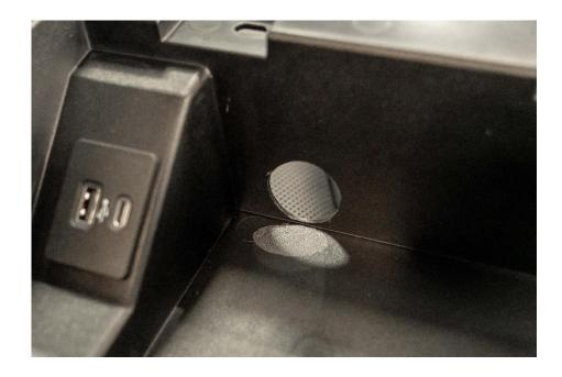
5. To gain access to remove the center console tray, lift up on the dash tray that sits above the radio as shown below. Remove the (2) 7mm bolts, you do not need to remove the tray, just lift up until the front clips release.
