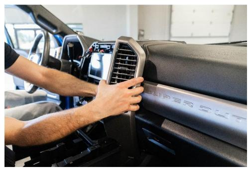
9. Once the vent pieces are removed, locate the (2) 7mm bolts at the bottom of the center stack, and remove them. This will allow removal of the small trim piece at the bottom.
