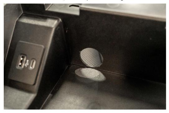
12. With the hole drilled, run the Edge CTS3's HDMI power cable from the OBD II port, under the dash, and up through the opening where the center console tray sits.
